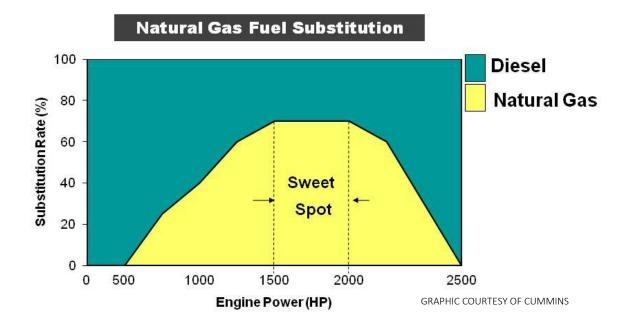
High Pressure Direct Injection (HPDI) is a means of introducing natural gas fuel directly into the combustion chamber at high pressure. Some amount of pilot fuel such as diesel is still needed for compression ignition. HPDI technology enables the use of higher proportions of gas, improving efficiency and further reducing emissions.
